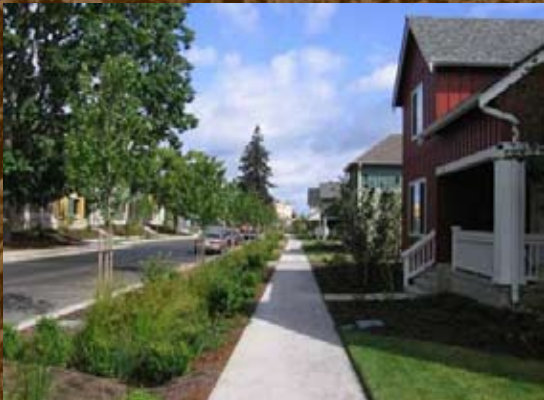
High Point uses compost-amended landscapes to manage stormwater.
